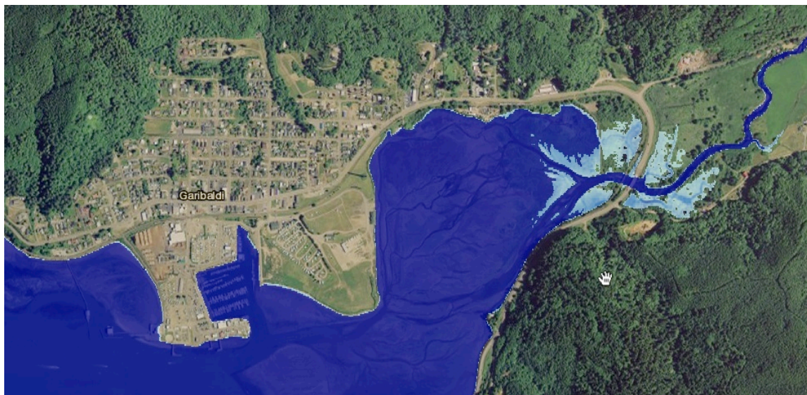
Figure 33: Projected inundation east of Garibaldi, OR assuming 2 ft/61 cm of sea level rise. Dark blue area represents current MHHW level at high tide. Light blue shading indicates additional inundation due to sea level rise.
